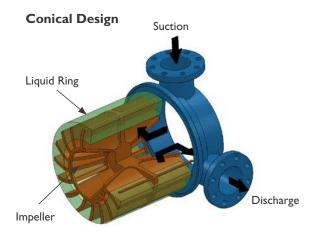
DEKKER liquid ring vacuum pumps are built to high quality standards and have the ability to handle large amounts of condensables. The condensing effect increases the actual pump capacity dramatically when handing saturated gas mixtures.
